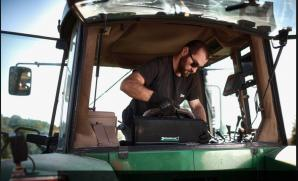
The new on-board tool set, measuring  $445 \times 270 \times 110$  mm (W x L x H), can be stowed behind or to the side of the driver's seat to save space, so it is always within easy reach.
