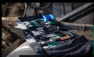
Everything at a glance: screwdrivers, offset screwdrivers, hammer, chisel, pipe wrench, side cutter, folding ruler, ring spanners, pin punches, magnetic torch, and a pocket knife.
