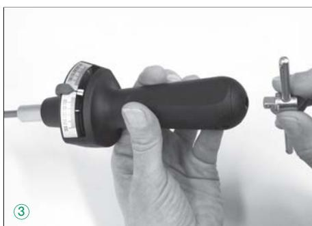
When the required value has been reached, the scale and the pointer must both be visible (this does not apply if measuring is carried out using the trailing pointer).
