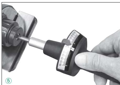
c) Position TORSIOMETER and apply force (see 3.) until pointer shows the required value ⑤.
