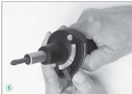
c) Position TORSIOMETER and apply force (see 3.) until the pointer reaches the pointer of the slide indicator ⑦.
