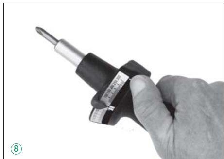
c) Before reusing the tool, slide the trailing pointer back to the starting position (see 4.3a).
