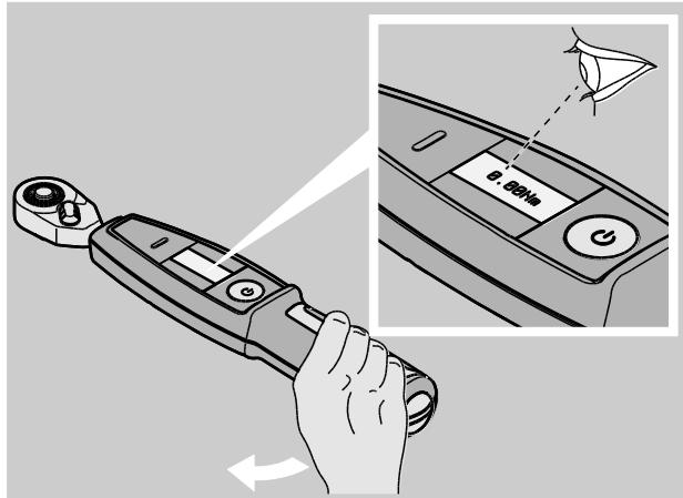
During the bolting process in "Track" function mode, the following displays and signals are provided depending on the settings which have been undertaken:
