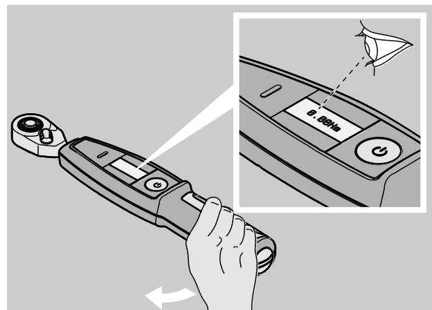
During the bolting process in "Peak" function mode, the following displays and signals are provided depending on the settings which have been undertaken:
